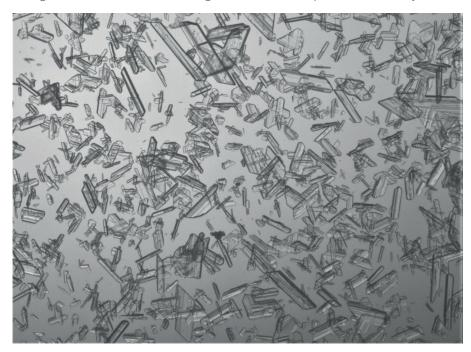
The uniform crystal size is another characteristic of Luxopharm® F 211. Carefully controlled growth allows production of single calcium sulphate dihydrate crystals with only a few twinned crystals. Medium crystal size is about 30  $\mu$ m.
