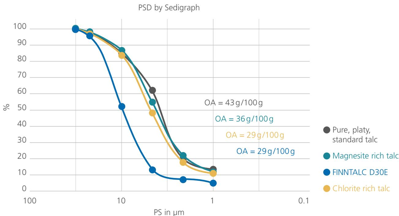
Figure 1: Particle size distribution of traditional types of talc and low oil absorption talc at the same fineness of grind (Hegman 4)
