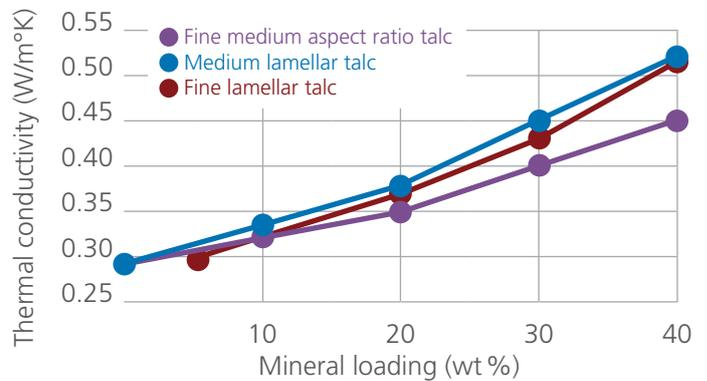
Figure 3: Thermal conductivity of PP compounded with talc
