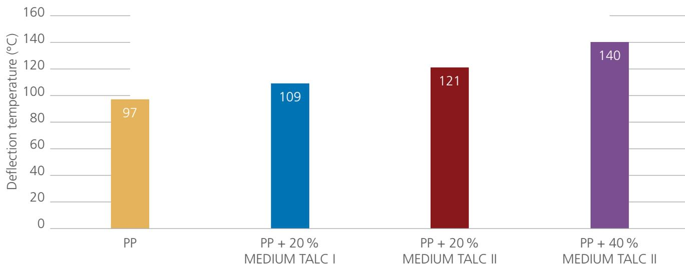
Figure 7: Deflection temperature of compounds with medium aspect ratio talc (I), high aspect ratio talc (II) and unfilled PP
