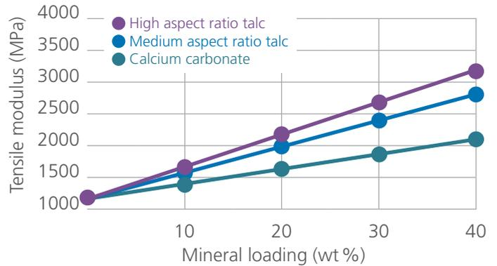
Figure 2: Stiffness of a PP compound with high aspect ratio talc, a mineral with medium aspect ratio, and calcium carbonate
