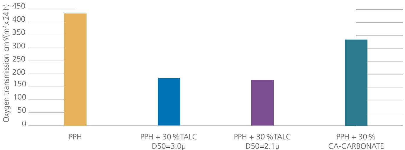
Figure 11: Reduced oxygen transmission in polyolefin food packaging by talc
