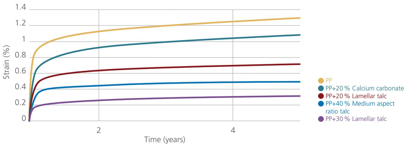
Figure 8: Creep of PP and filled polypropylene
