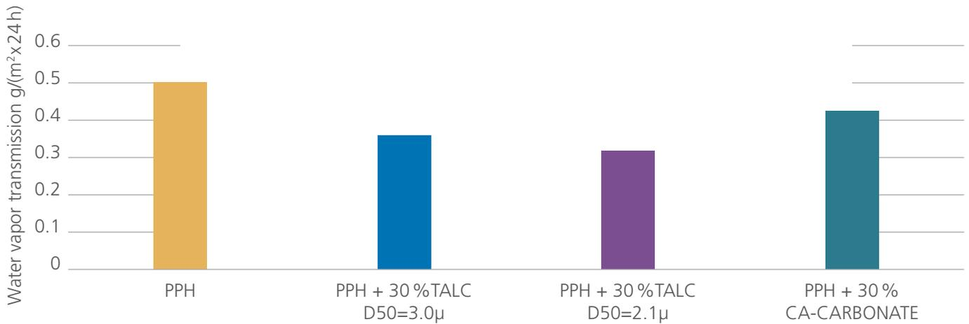
Figure 10: Reduced water vapor transmission in polyolefin food packaging by talc
