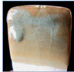
Standard (Discolored & Poor Sag)
