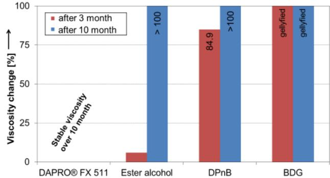
Data displayed are showing that only with DAPRO FX 511 stable viscosities could be achieved in a silicate based paint. The use of all other tested coalescents resulted in a tremendous viscosity rise.
