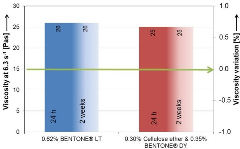
BENTONE® LT is a grade which could be as a stand alone alternative to a combination out of cellulose ether and Xanthan gum. BENTONE® DY is typically formulate as a partial replacement for cellulose ether.
