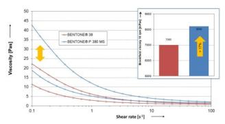
The results show that at equal active clay content the viscosity of an alkyd-based coating system that incorporates BENTONE® P 380 MS will be substantially higher at lower and medium shear rates than one which uses a conventional organoclay pregel. Tests showed that other properties of the coatings, e.g. sag resistance, were improved significantly and without any negative impact on flow properties.
