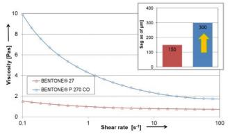
Comparing the sagging stability provided by both samples clearly displays that with the use of BENTONE® P 270 CO a significant improvement can be achieved.
