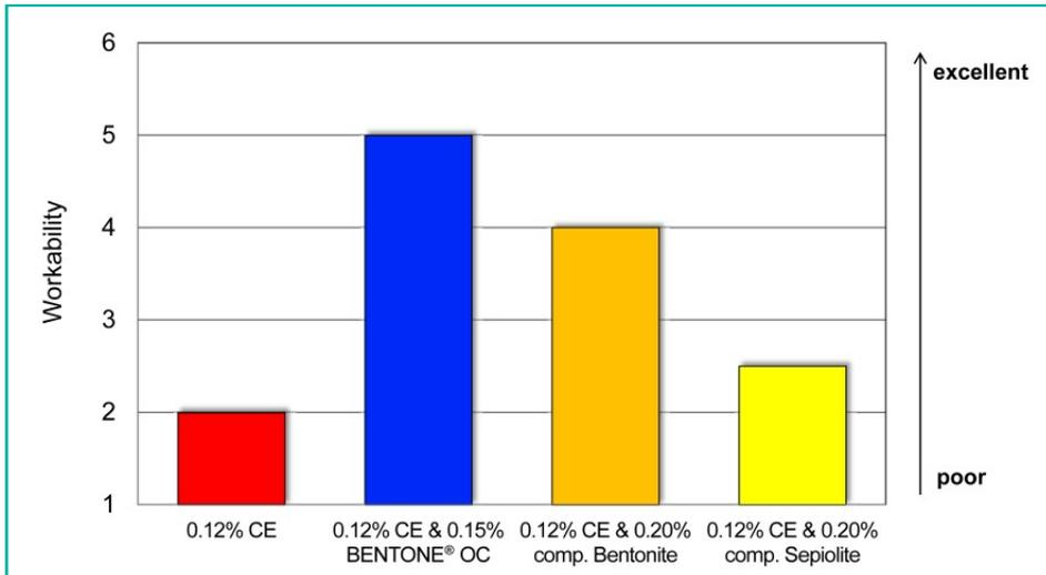
The use of BENTONE® OC results in the best application properties and the least stickiness on the tool. Both competitive clays provide less good performance, even when used in higher concentrations compared to BENTONE® OC.
