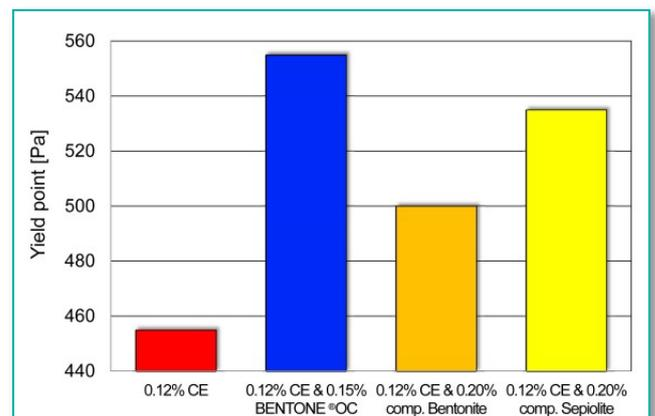
The highest sag stability and yield points are obtained with BENTONE® OC, both compared to competitive clays as well as to the formulation with cellulose ether only. This means thicker stable layers can be applied on the vertical surface without sagging.
