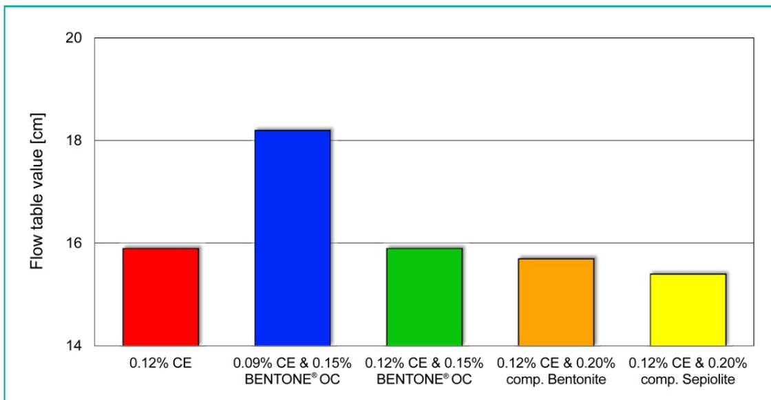
For all clay additives equal spread rates of around 16 cm are observed when formulated with an equal amount of 0.12% of the original cellulose ether content. The sample with lower cellulose ether content demonstrates significantly lower consistency and is therefore not of practical use.
