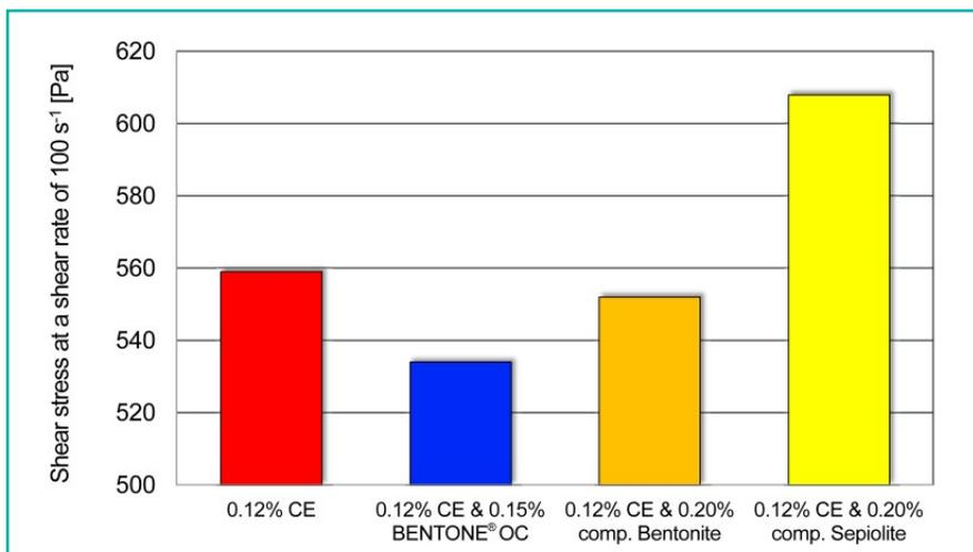
The formulation with BENTONE® OC requires the lowest amount of energy to initiate flow at a shear rate of  $100 \text{ s}^{-1}$ . The competitive Bentonite grade shows also better results in comparison to the formulation with cellulose ether only. The competitive Sepiolite, shows even poorer results than the formulation with cellulose ether only.
