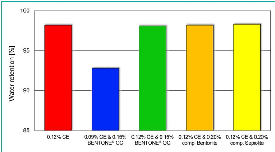
All formulations with the initial concentration of cellulose ether show the required high water retention values. With reduced cellulose ether content, significantly lower water retention values are obtained. This can not be compensated by the addition of BENTONE® OC. Due to these results, the formulation with reduced cellulose ether content can not be considered for further evaluation.
