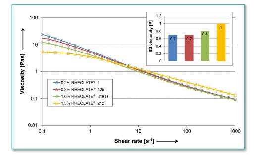
RHEOLATE<sup>®</sup> 212 provides the highest viscosities at high-shear rates and the most Newtonian flow character. Both ASE grades, RHEOLATE<sup>®</sup> 1 and RHEOLATE<sup>®</sup> 125, act most shear thinning. The sample equipped with RHEOLATE<sup>®</sup> 310 D performs in between.
