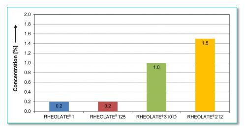
Both tested acrylic thickeners, RHEOLATE<sup>®</sup> 1 and RHEOLATE<sup>®</sup> 125 require by far the lowest loadings to achieve the required Brookfield viscosity. RHEOLATE<sup>®</sup> 212, providing Newtonian flow characteristics, needs the highest concentrations.
