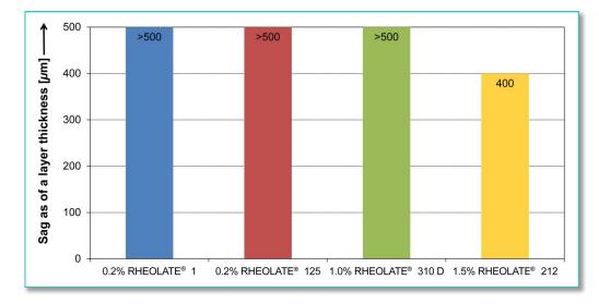
Samples formulated with both ASE grades, RHEOLATE<sup>®</sup> 1 and RHEOLATE<sup>®</sup> 125, as well as RHEOLATE<sup>®</sup> 310 D demonstrate the highest sag stabilities with applicable layer thickness of above 500  $\mu$ m. The sample made with the Newtonian acting NiSAT grade RHEOLATE<sup>®</sup> 212 was stable up to a layer thickness of 400  $\mu$ m.
