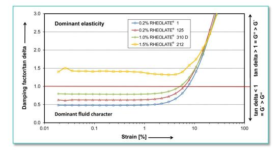
Samples formulated with both ASE grades, RHEOLATE<sup>®</sup> 1 and RHEOLATE<sup>®</sup> 125, display the highest elasticities. RHEOLATE<sup>®</sup> 310 D gave somewhat lower elastic properties. Only the use of RHEOLATE<sup>®</sup> 212 results in a shift to dominant fluid behavior at lower strain values.
