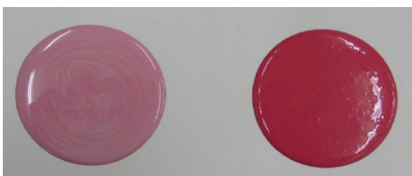
Figure 5: Left - improper emulsification of the colorant into the base paint Right - problem solved by adding a polyphosphate emulsifier (NUOSPERSE® FA 196)
