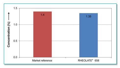
RHEOLATE<sup>®</sup> 658 requires slightly lower quantities to achieve the required KU viscosity. This indicates a slightly higher efficiency in comparison to the tested market reference NiSAT product.
