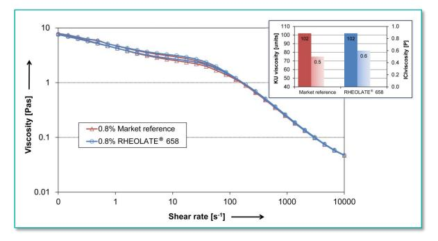
RHEOLATE<sup>®</sup> 658 is matching the flow characteristics of the tested market reference NiSAT thickener exactly at equal mid-shear viscosity. The high-shear/ICI viscosity shows only marginal differences between the two products.
