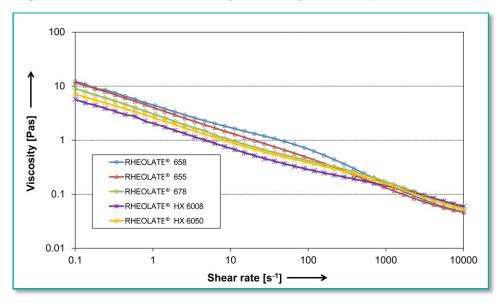
Figure 1: Flow characteristics - Styrene - Acrylic PVC 50 paint
