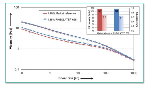
The use of RHEOLATE<sup>®</sup> 658 results in similar flow characteristics than the market reference NiSAT when adjusted to equal KU viscosity. The detected hysteresis area in the graph plotted is in only slightly lower with RHEOLATE<sup>®</sup> 658. This indicates a slightly quicker recovery of the viscosity after removal of shear forces.
