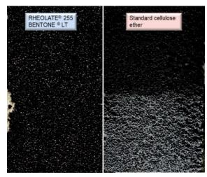
For this test a system filled with black quartz was chosen due to the typically strong sensitivity to this effect after exposure to high humidity conditions.
